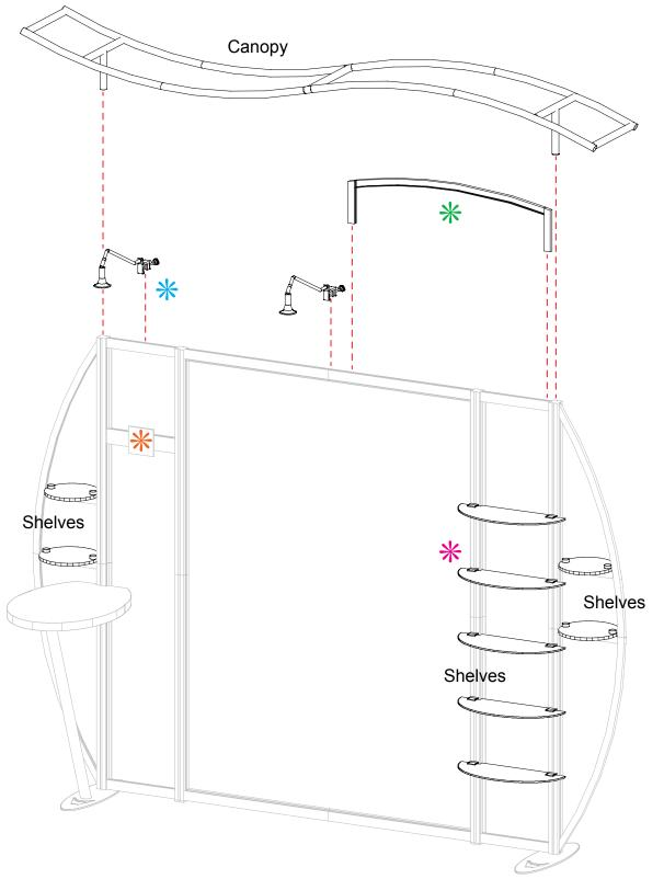
WHEN DISASSEMBLING ALUMINUM EXTRUSION, TIGHTEN ALL SETSCREWS AND LOCKS TO PREVENT LOSS DURING SHIPPING
