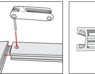
**Extrusion & Lock Connection**
