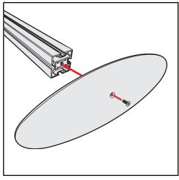
Base Plate & Extrusion Connection
